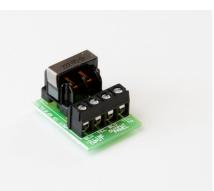
The ACT 4425 iD Line Filter is designed to connect between the BLUE and YELLOW data wires and the input terminals of the alarm control panel. The filter allows data to pass through normally but prevents RFI entering the control panel. The ACT 4425 should be fitted to all ID systems, especially on take-overs where existing wiring has been used, to prevent potential false alarms from occuring.
